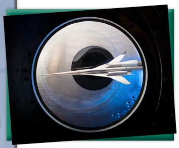
The window in the sidewall of the 8-by-6 foot supersonic wind tunnel at NASA's Glenn Research Center shows a 1.79 percent scale model of a future concept supersonic aircraft built by The Boeing Company
